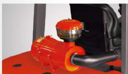
Pre-cleaner engine air intake
