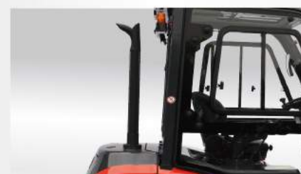
Upward Exhaust Pipe I
