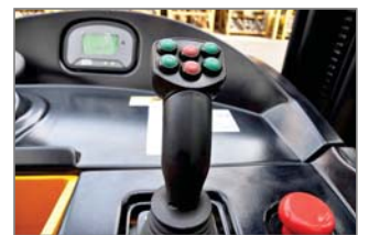
Control handle with integrated thumb stick, allows smooth operation of (1)Tracel, (2) Lift / low (3) Controls Tilt and Fork Reach.
